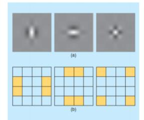
Fig 3 Typical wavelets associated with the 2-D separable DWT
